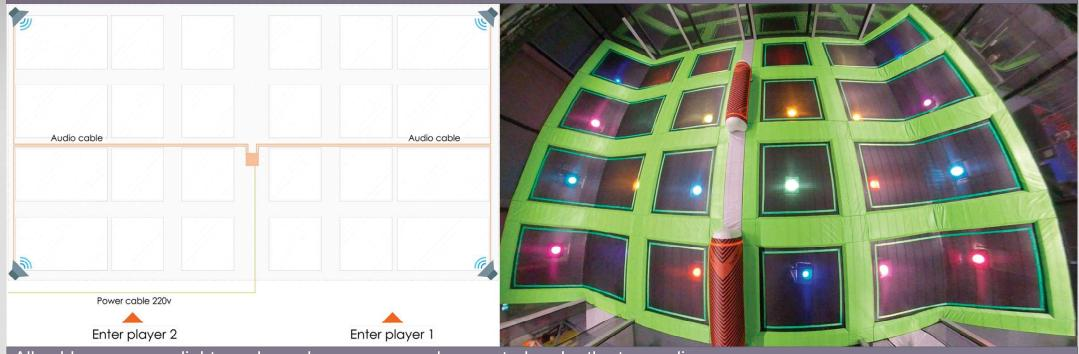
All cables, sensors, lights and speakers are securely mounted under the trampolines.
